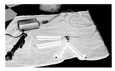
In the photo above, the "tea bag" is the white mesh wine-fermenting bag underneath the pump, tubing and bubbler stones. The black cylinder is an aquarium heater.
